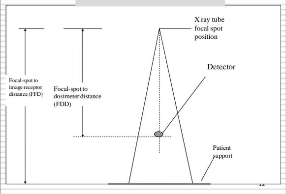
The x-ray tube output was determined as the ratio of average dosimeter reading (in air kerma) to the tube current-time product used for tube voltages 50-110 kVp in steps of 10 kVp . The values of the x-ray tube output per mAs were plotted against the tube potential and the resulting curve was fitted using a power function.
